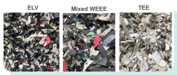
Figure 38. Examples of shredded fractions that make up the input of specialised WEEE and ELV recyclers.
