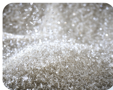
Figure 50: Close-up of pellet crystals produced by a dissolution recycling process.
