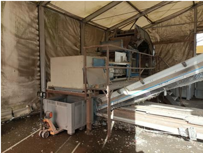
Figure 12 Preshredder treatment of smaller material fraction. Left: Magnetic separator. Right: additional sorter.
