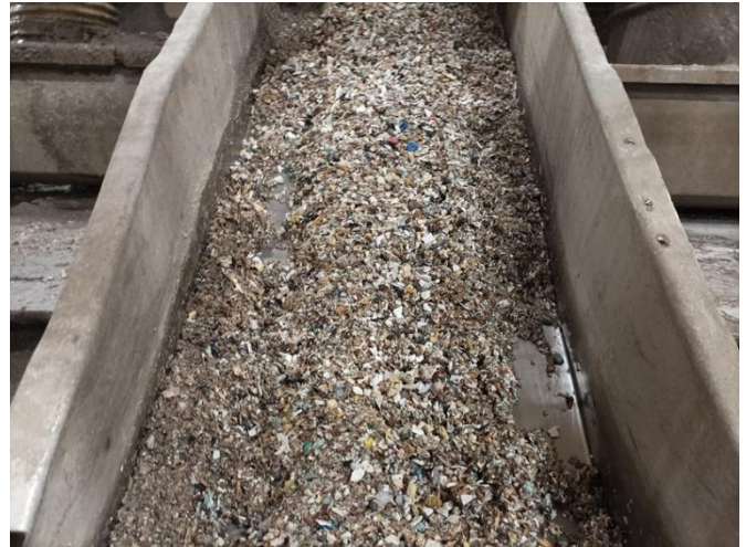
Figure 24 Left: wet grinding and density separation equipment. Right: material separated from the waste stream through density separation equipment.
