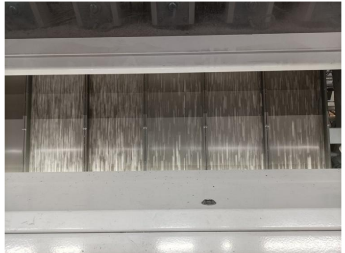
Figure 26 Left: Electrostatic sorting equipment. Note the presence of cleaning equipment to prevent the spread of microplastics. Right: colour sorting equipment.
