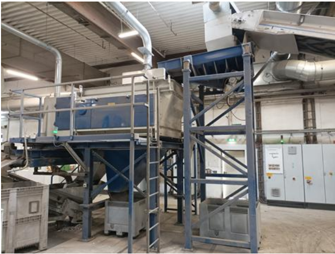
Figure 16 Eddy current separation. Left eddy current separator. Right: material removed from waste stream.
