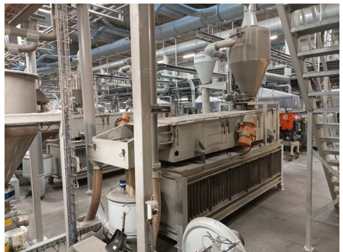
Figure 27 Left: extrusion with melt filtration equipment and operator cleaning in between the melt filter change cycles. Right: the active pellet cooling equipment.
