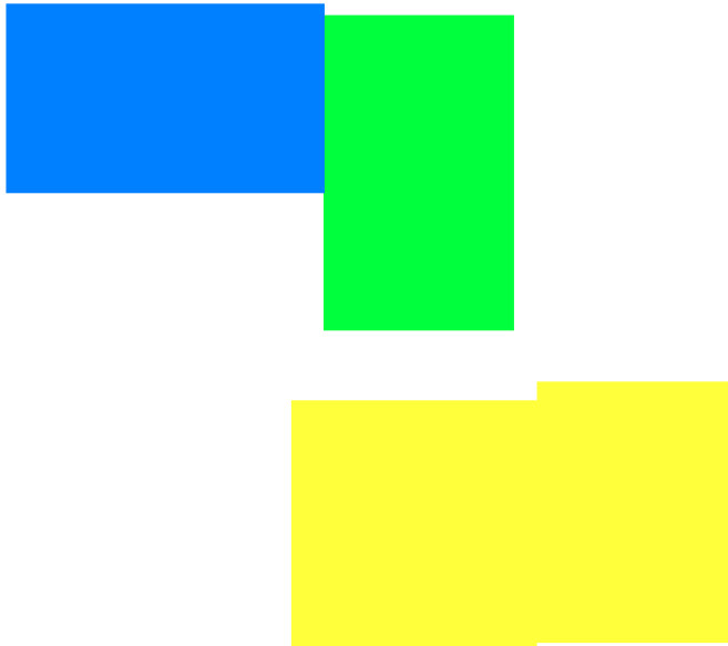
Figure 20 Plant C Layout. Blue is outdoor area for receiving & shredding of profile waste; green is indoor building where mechanical processes occur; yellow is indoor building where regrind is extruded with melt filtration to produce pellets; with outdoor silo storage or packaged good storage under canopy.
