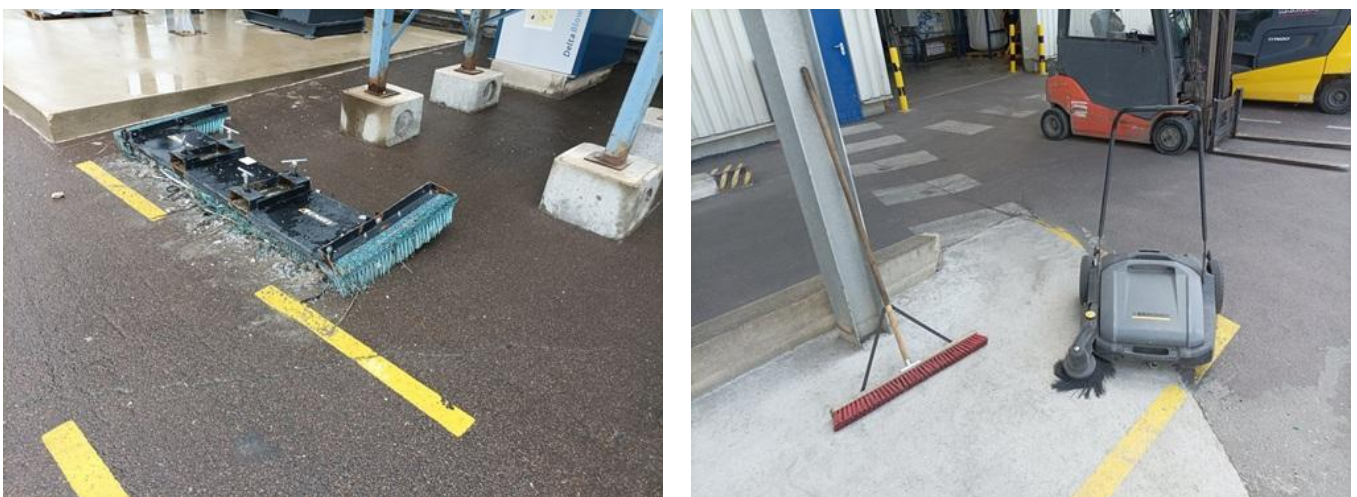
Figure 8 Cleaning equipment used to control spread of microplastics on site. Left: forklift mountable brushes. Right: broom and mechanical sweeping and collection equipment.
