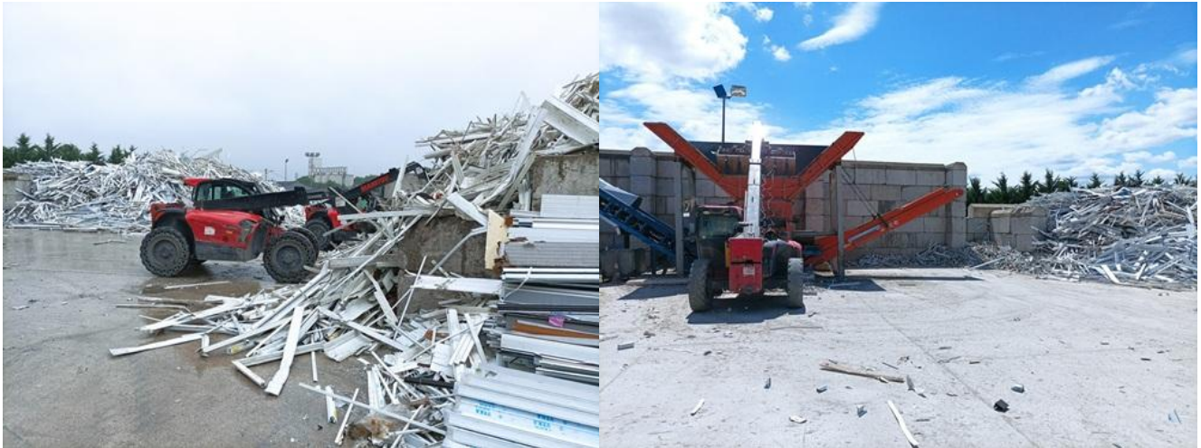
Figure 3 Line Input Operator feeding outdoor shredder. Left: collection of profile waste. Right: feeding the first shredder.
