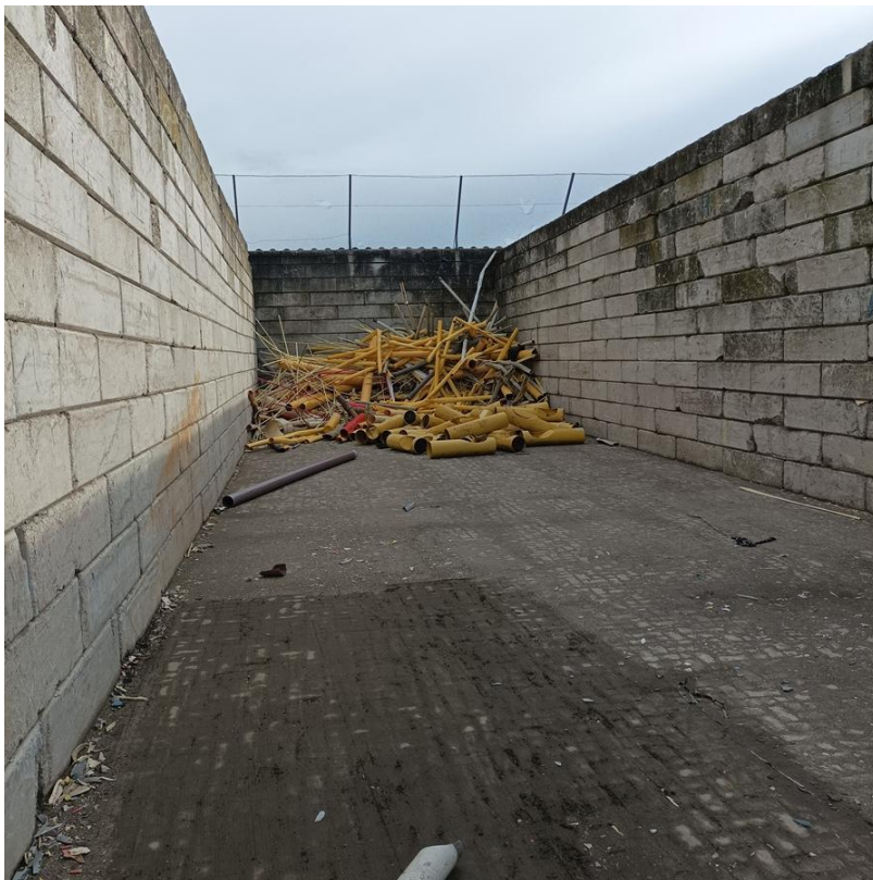
Figure 35 One of the smaller bunkers of Plant D with a batch of post-consumer industrial pipes. Note the fencing/netting installed on top of the bunker wall.
