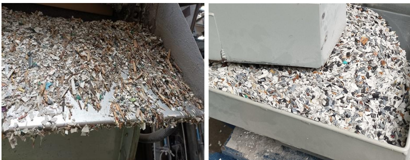
Figure 5 Left: Waste output of the density separation step. Right: Construction profile regrind before final mechanical processing in plant A.
