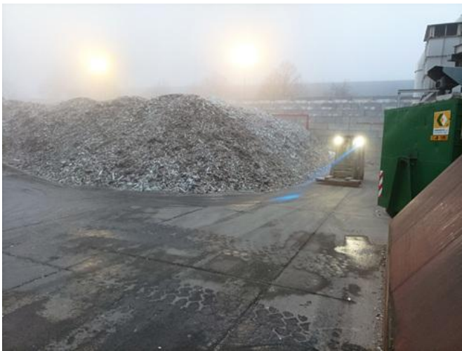
Figure 29 Forklift mounted brushes employed by Plant C. Left, a forklift in operation cleaning the passage ways between the stored waste and the feeding equipment. Right, a close up of the mountable brushes.
