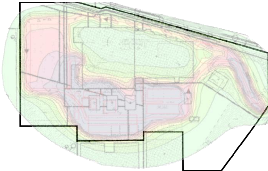
Figure 19 plant outline with superimposed dust deposition modelling results. The outer most green section is indicative of a deposition of between 10.5 and 21 \text{ mg/m}^2/\text{d} while the inner most dark grey represents a deposition of >105 \text{ mg/m}^2/\text{d} .
