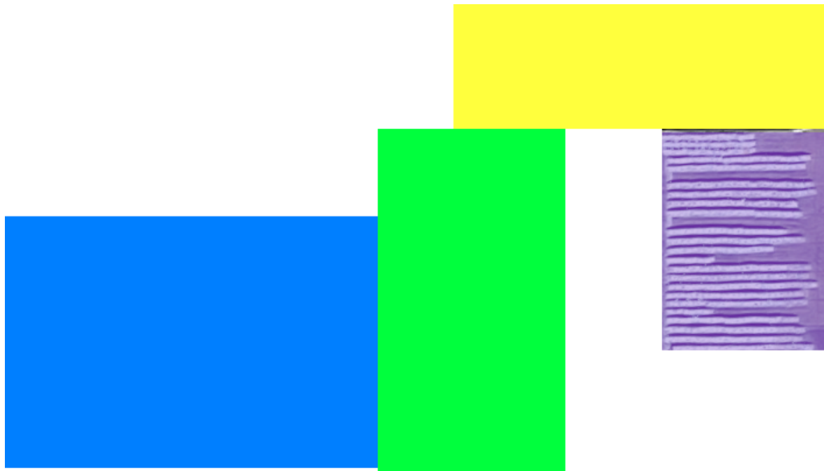
Figure 1 Plant A Layout. Blue is outdoor area for receiving of profile waste; green is indoor building where mechanical processes occur; yellow is indoor building where regrind is extruded with melt filtration to produce pellets; sealed big bags of finished product is stored in an outdoor area (purple). Office buildings not shown.
