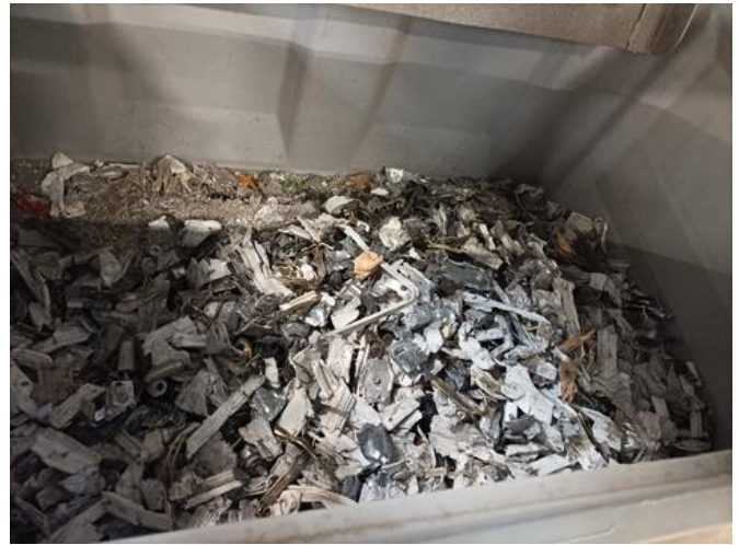
Figure 16 Eddy current separation. Left eddy current separator. Right: material removed from waste stream.
