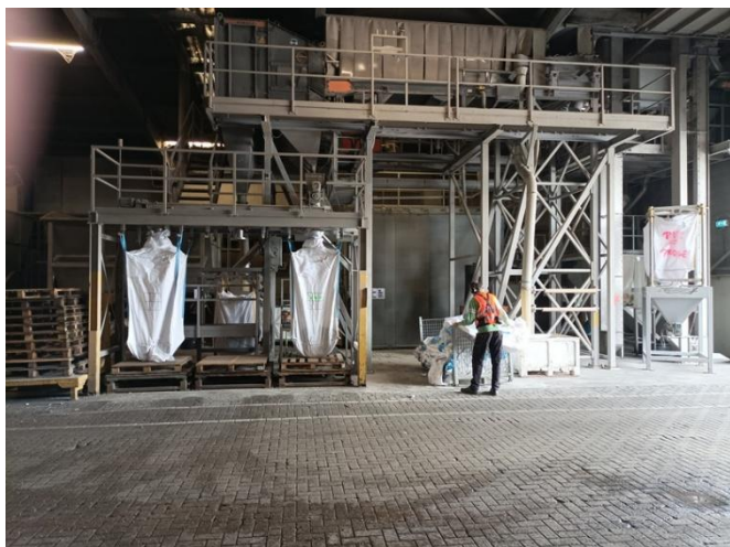
Figure 33 Left: big bag feeding station of the grinding hall. Right: Operator performing visual check of grinder input.
