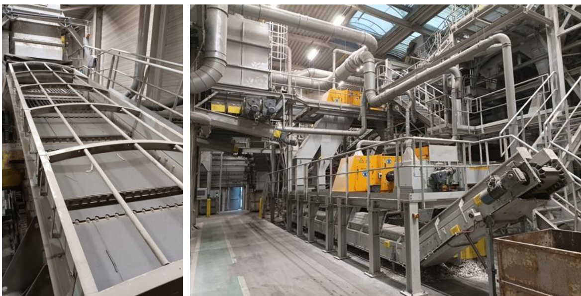
Figure 23 Left: Sieve System. Right: the first mechanical sorting system for the three size fraction streams.
