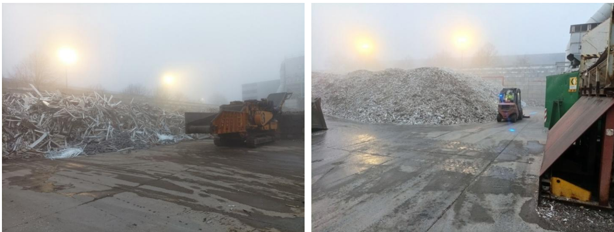
Figure 21 Left: outdoor storage area for construction profile waste as received with the first mobile outdoor shredder. Right: shredded waste and the hopper that starts the conveyer chain for the indoor processing. Note the forklift truck on the right is equipped with a brush to clean the surface and prevent spread of material to other areas of the plant and beyond.
