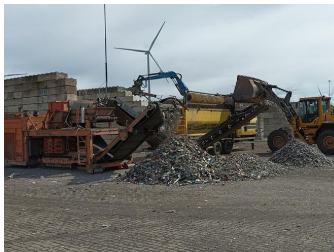
Figure 32 Left: crane feeding outdoor shredder. Right: output fractions of the outdoor shredder.
