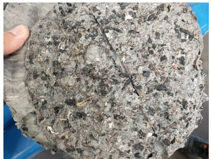
Figure 6 Left: Extruder equipped with melt filtration, Right: Typical filter cake showing impurities captured on a metal sieve during melt filtration.
