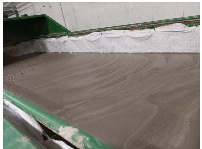
Figure 25 Left: Process water cleaning system and reagents used to in the process. Right: sludge which is mainly the mineral impurity removed from the waste stream.
