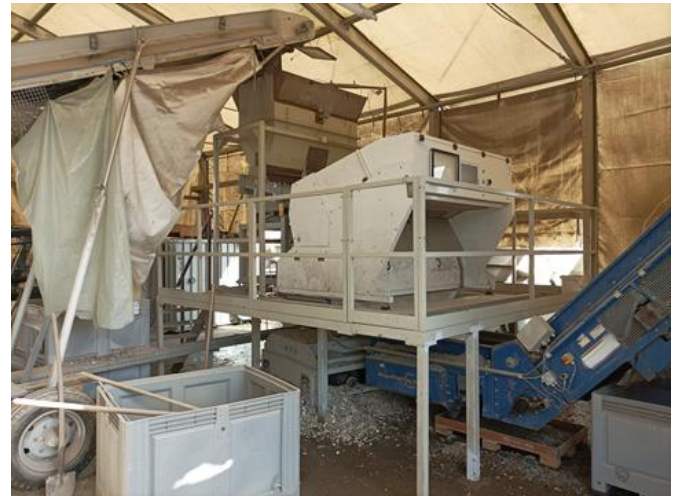
Figure 12 Preshredder treatment of smaller material fraction. Left: Magnetic separator. Right: additional sorter.
