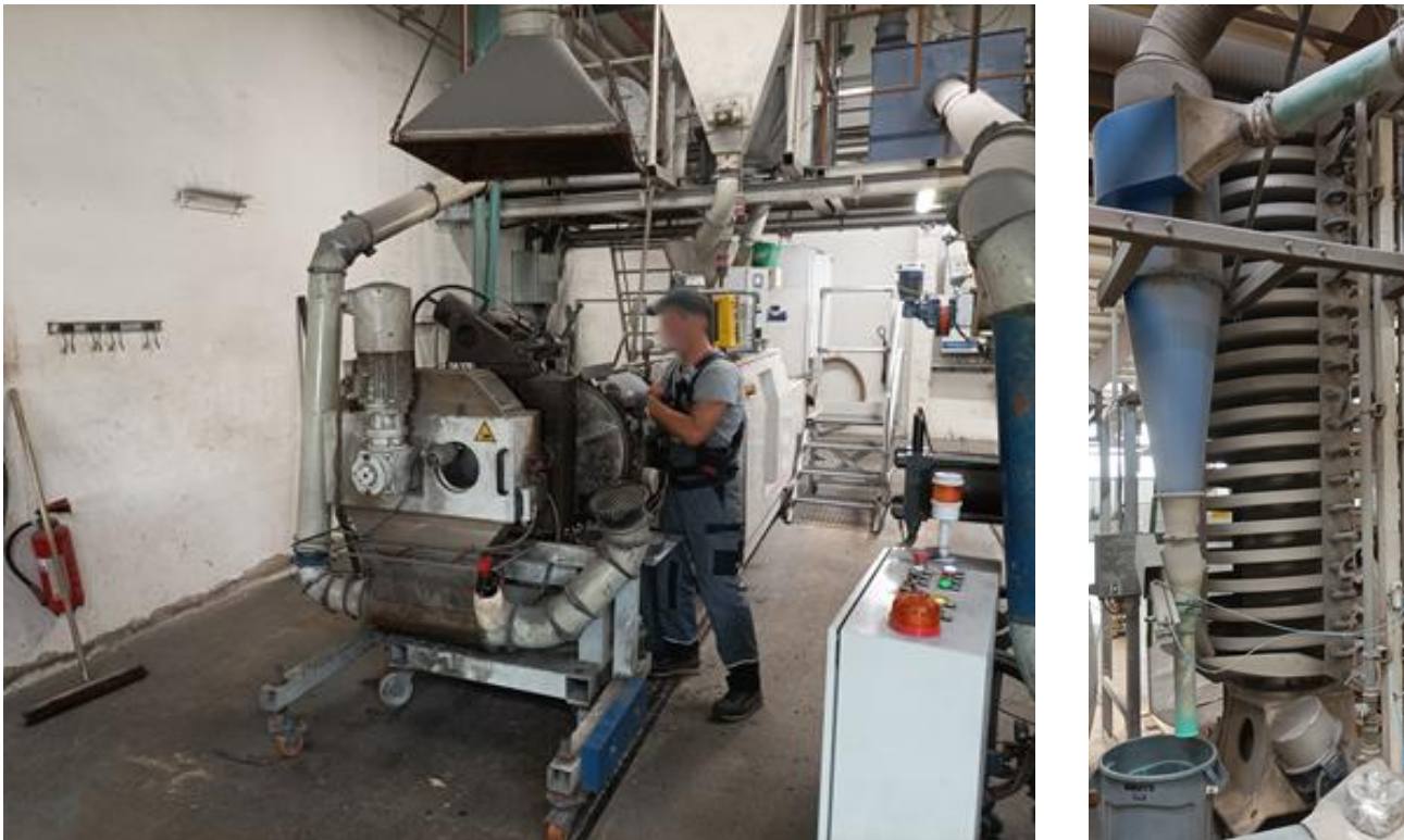
Figure 18 Equipment in Extrusion Hall. Left: Extrusion equipment with Melt-Filtration. Right: pellet cooling tower.
