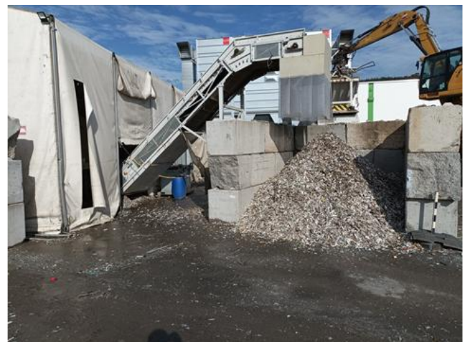
Figure 13 Main output of the pre-shredder process. Left: larger profile pieces being shovelled into the indoor shredding process. Right: the finer output of the pre-shredder processing ready for introduction into the indoor mechanical process.
