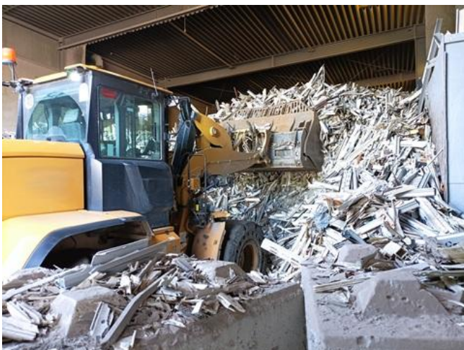
Figure 13 Main output of the pre-shredder process. Left: larger profile pieces being shovelled into the indoor shredding process. Right: the finer output of the pre-shredder processing ready for introduction into the indoor mechanical process.
