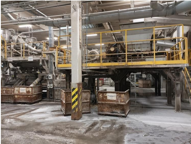
Figure 24 Left: wet grinding and density separation equipment. Right: material separated from the waste stream through density separation equipment.
