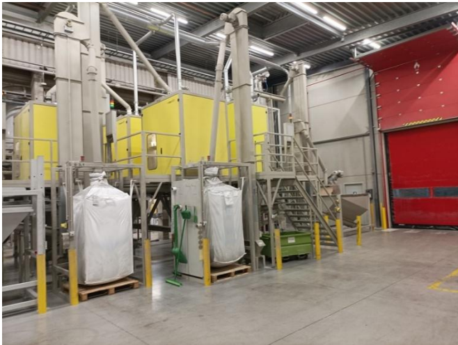
Figure 26 Left: Electrostatic sorting equipment. Note the presence of cleaning equipment to prevent the spread of microplastics. Right: colour sorting equipment.
