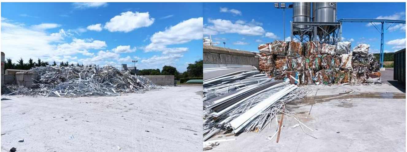
Figure 2 Stored construction profile waste. Left: predominantly post-consumer material. Right: more pre-consumer material.
