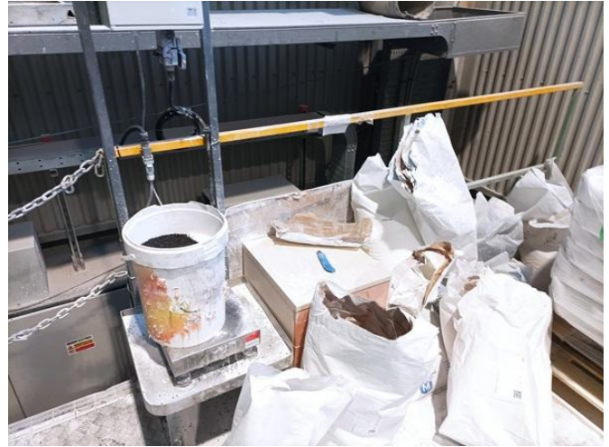
Figure 7 Compounding step. Left: compounding vessel with main raw material feed being regrinded material from silo that can be seen on the left side of the picture. Right: solid additive weighing station.
