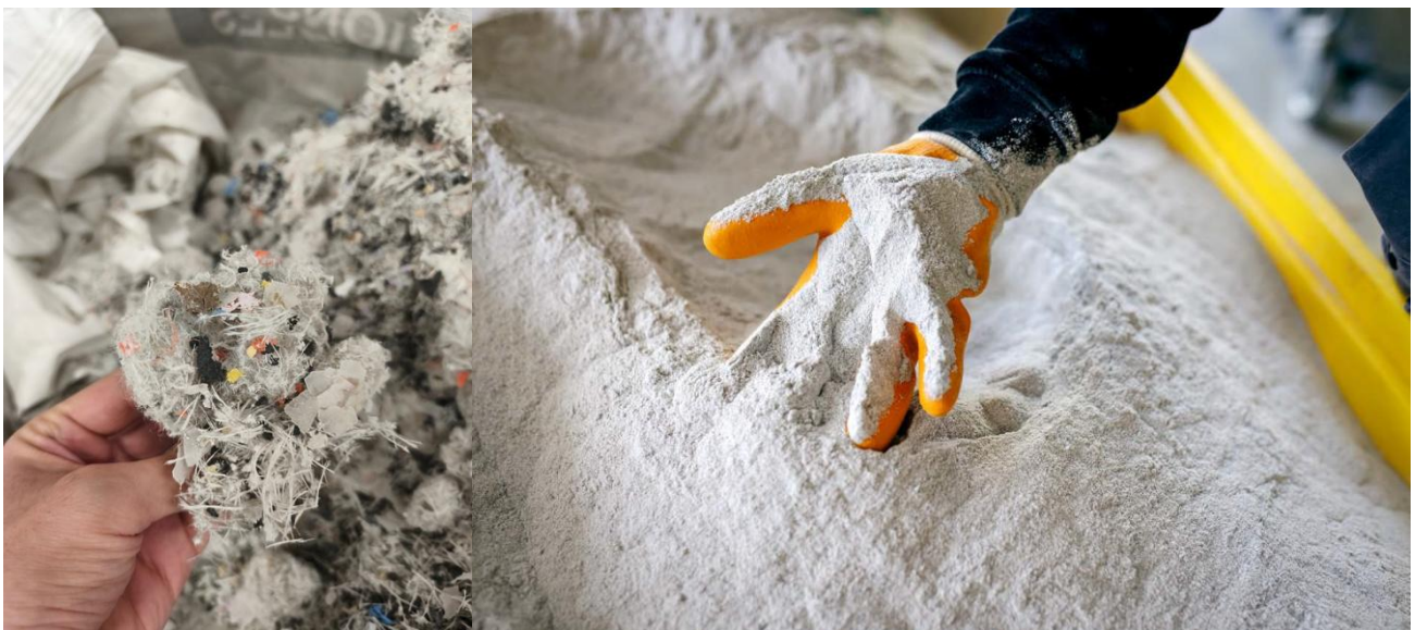
Figure 19 Left: PET fibres making up the bulk of the waste output from the sieving step. Right: micronized flexible PVC recyclate.
