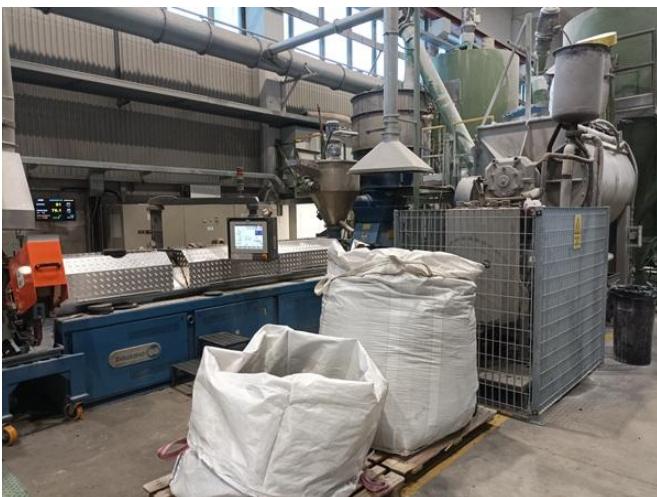
Figure 8 Extrusion equipment. Left: shows compounding vessel from other side and the first part of the extruder. The big bags shown are where workers deposit filter cakes and spent metal mesh filters. Right: end of the extrusion line with a clear view of the melt filtration unit and the pipe transporting the pellets to the cooling station.
