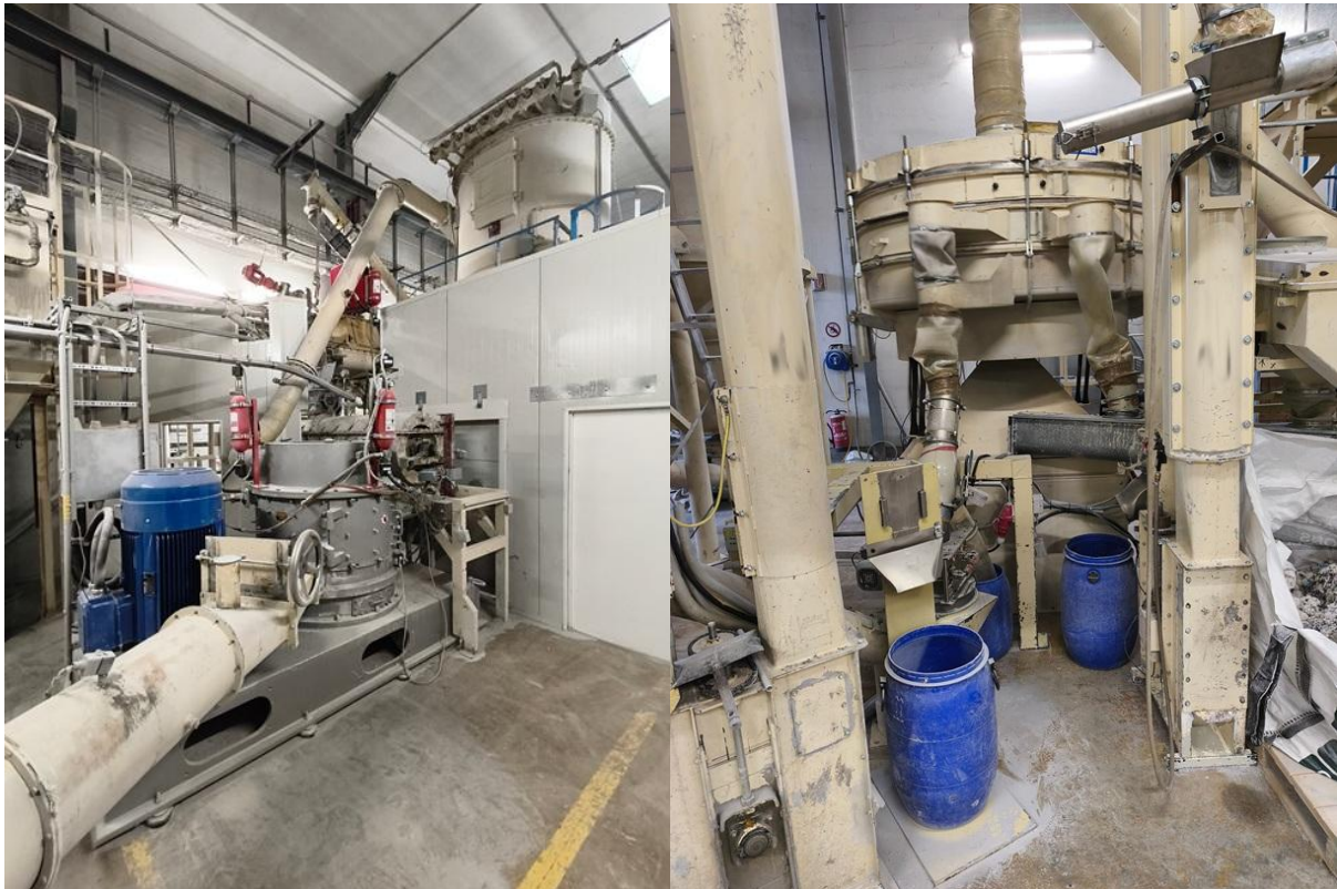
Figure 18 Left: cryogenic grinder. Right: industrial sieve.
