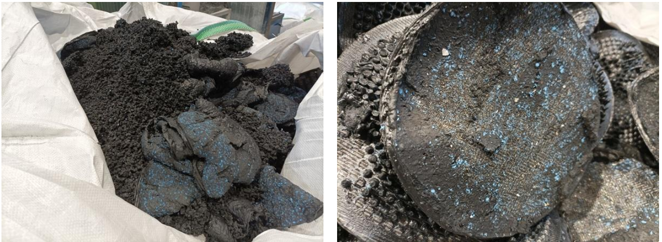
Figure 9 Residues from the melt filtration process. Left: filter cakes and Right: metal mesh filters.
