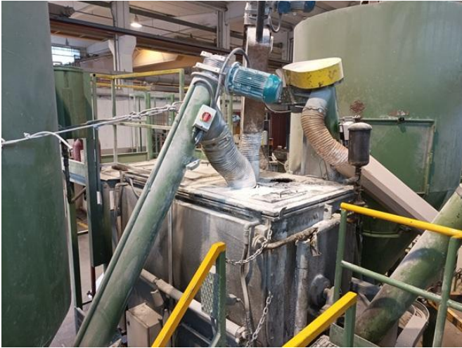
Figure 7 Compounding step. Left: compounding vessel with main raw material feed being regrinded material from silo that can be seen on the left side of the picture. Right: solid additive weighing station.
