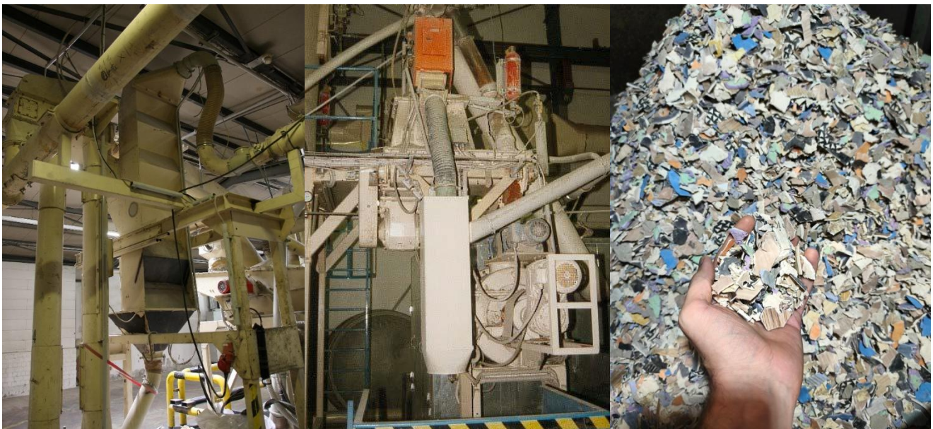
Figure 17 Left: Wind sifter. Middle: metal separation. Right: resulting flexible flooring material.
