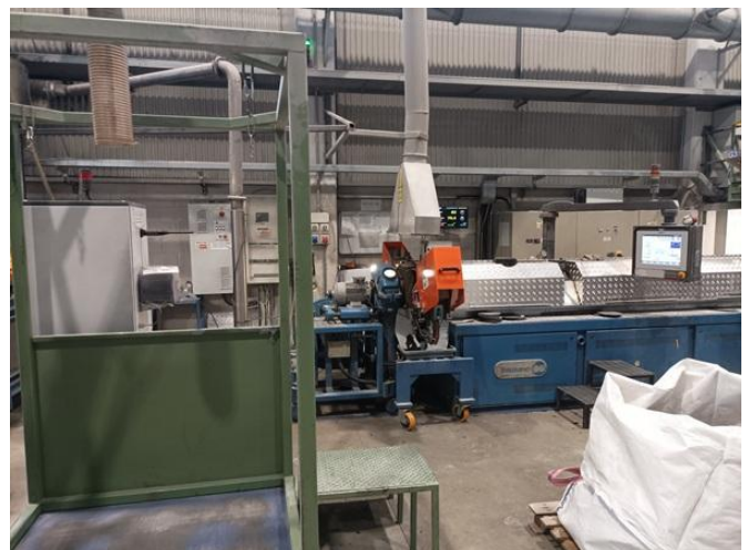
Figure 8 Extrusion equipment. Left: shows compounding vessel from other side and the first part of the extruder. The big bags shown are where workers deposit filter cakes and spent metal mesh filters. Right: end of the extrusion line with a clear view of the melt filtration unit and the pipe transporting the pellets to the cooling station.
