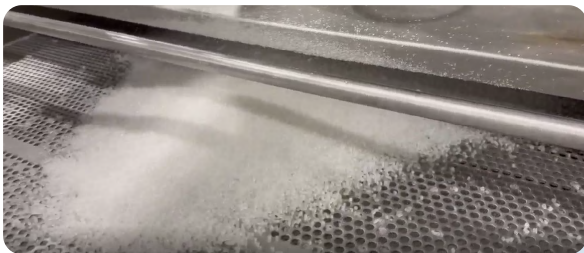
Figure 49: Close-up of a classifier used in dissolution recycling for separating particles after the dissolution process.
