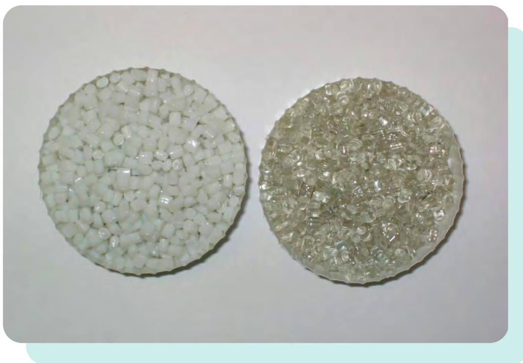
Figure 30. Left: Crystallised PET flakes, right: Amorphous PET flakes
