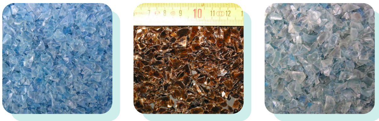
Figure 29. Left to right: sorted blue, brown and light blue PET flakes
