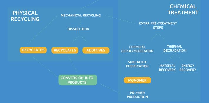
The most common and widely established is mechanical recycling, which falls under physical recycling. Via a mechanical operation, plastic waste is most often grinded, washed, dried, extruded, re-granulated and then converted. Physical recycling also includes solvent-based purification, such as dissolution processes. Today, physical recycling technologies contribute the most towards the EU recycling rates.
