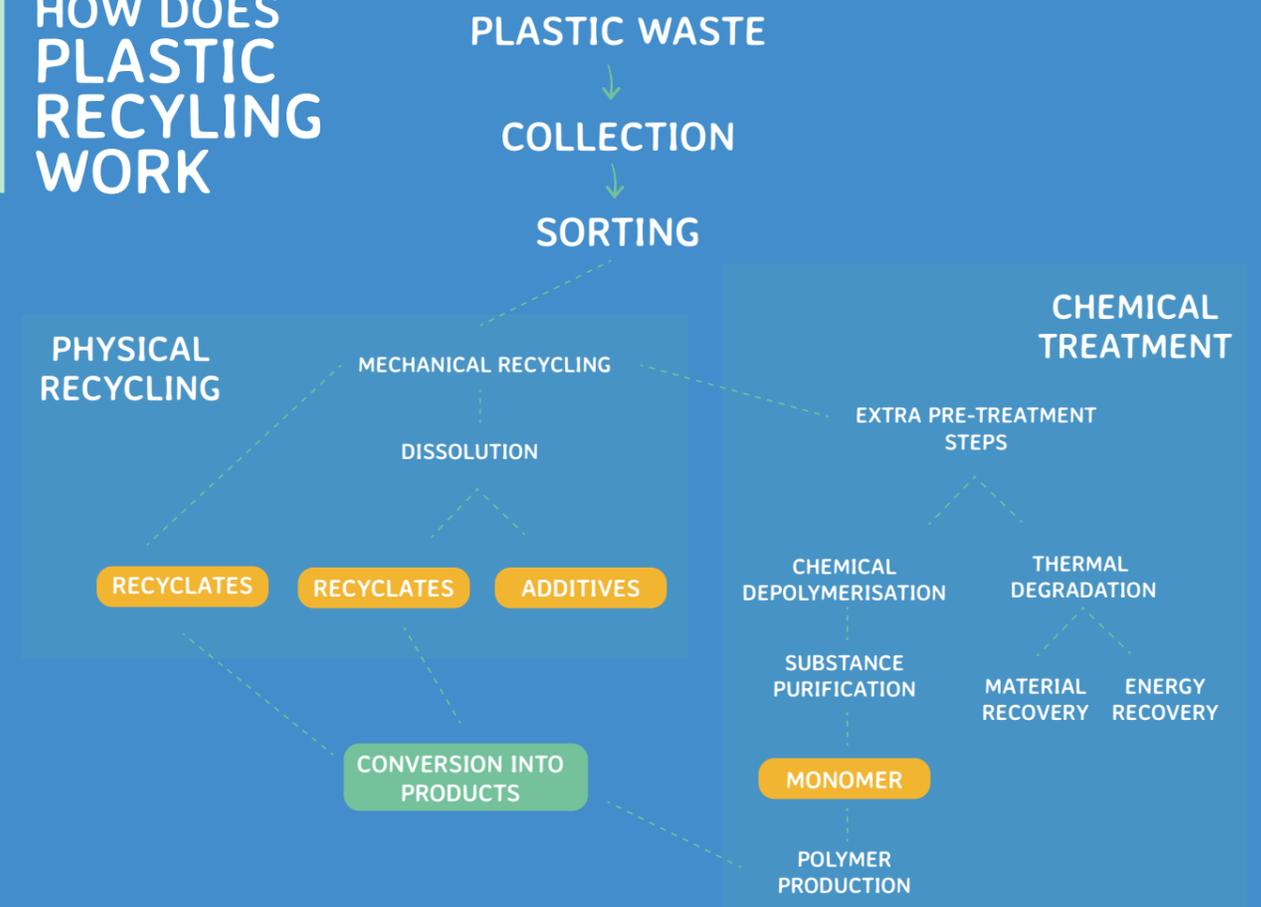
The most common and widely established is mechanical recycling, which falls under physical recycling. Via a mechanical operation, plastic waste is most often grinded, washed, dried, extruded, re-granulated and then converted. Physical recycling also includes solvent-based purification, such as dissolution processes. Today, physical recycling technologies contribute the most towards the EU recycling rates.
