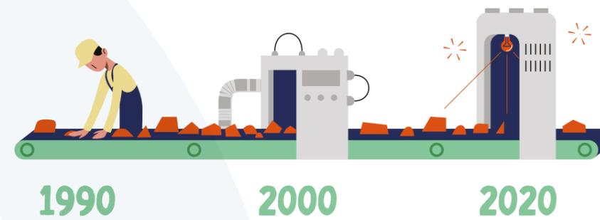
Near Infra-Red (NIR) technology is used to separate plastics
